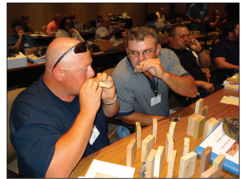
A hands-on demo: Dip a small piece of red oak in soapy water and then blow on the other end. Bubbles will form on the wet end. Cool, huh?
